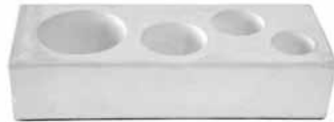
2| mould of 4 half-bowls for inside re-shaping
