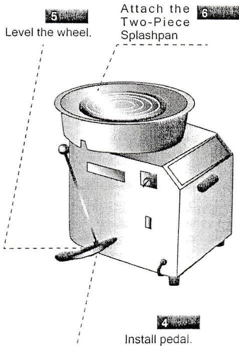
6. Attach the Two-Piece Splashpan to the wheel, seating it under the flange of the bearing holder (under the wheelhead)
