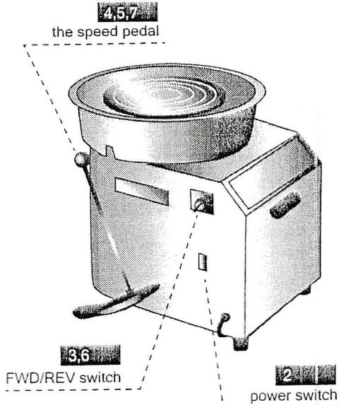
7. DO NOT change rotation direction while motor is running. Do so only after wheelhead has come to a complete stop.
