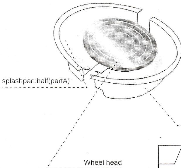
1. Insert splashpan half (part A) into the groove (recess) on the bottom of the bearing holder.
